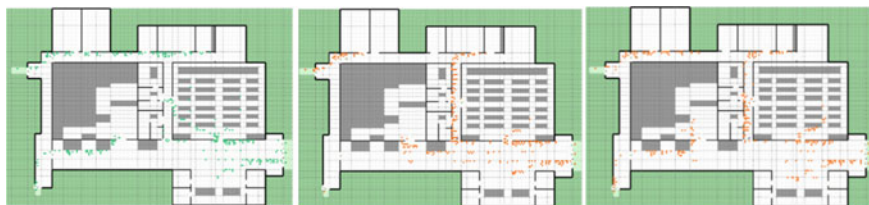
Fig. 10 Evacuation route patterns: if the occupants are familiar with the building (left); the occupants do not follow the guiding signage (middle); the occupants follow guiding signage (right)
