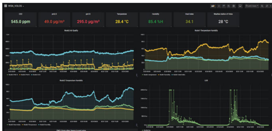
Fig. 5 Dashboard that shows latest measurements on top and plots with time-series values for two consecutive days
