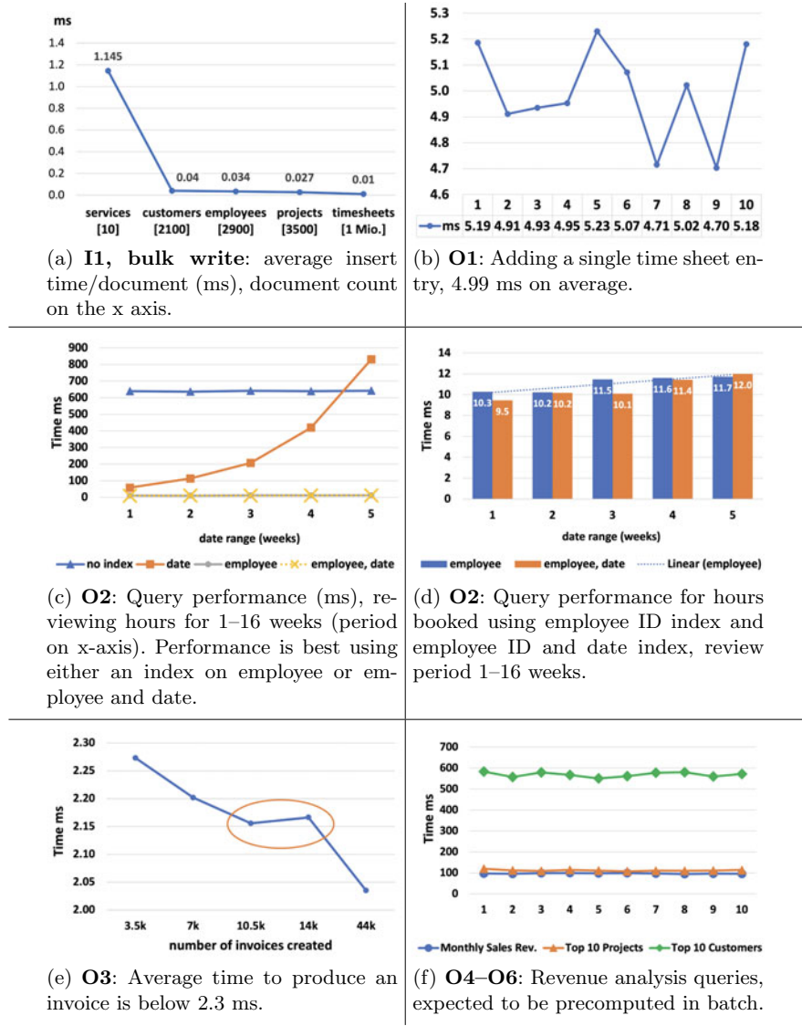
Fig. 2 Performance. In I1 the leftmost item (services) is the highest although the data volume is the smallest, as a new collection is created and the creation time is not amortised over the number of services. Another reason could be that it is a cold run. O2: EmployeeID index and employeeID and date index perform similarly. O3: Paging starts when more than 3 months’ worth of invoices are to be created. The ellipse highlights the area where we allow paging. O4–O6: Two queries are fast enough (0.1 ms), and one is slower: candidate for batch
